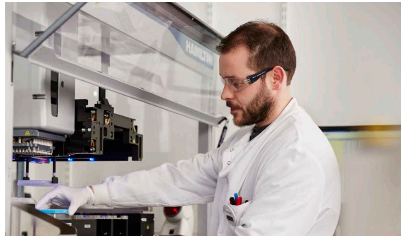
A Clinical Scientist starts the TGS process on a Hamilton Microlab STAR Robot.
